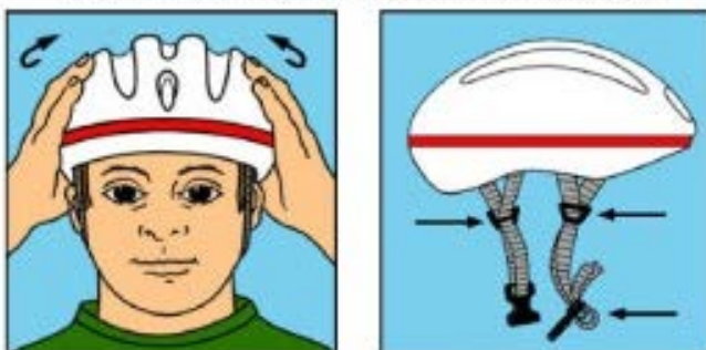
Make sure the helmet fits snugly and does not obstruct the field of vision. Make sure the chin strap fits securely and that the buckle stays fastened.
